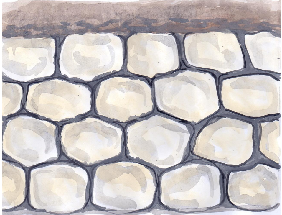
Illustration 33: Lay stones as closely and tight-fitting as possible
