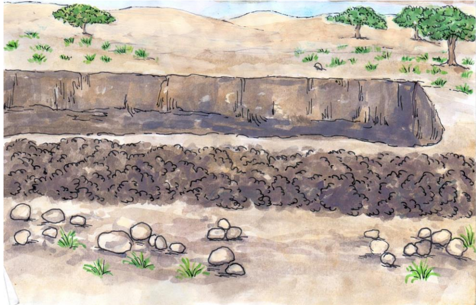
Illustration 42: Don't leave excavated soil downstream
