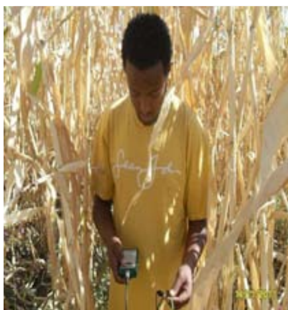
Figure 3.10: Moisture reading using Watermark digital data logger from buried monitoring electrodes
