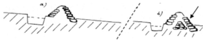
Figure 9: Double faced stone/soil bunds with collection trench
