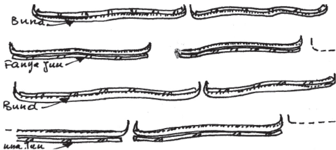
Figure 20: Combination of Fanya juus and soil bunds along the slope
