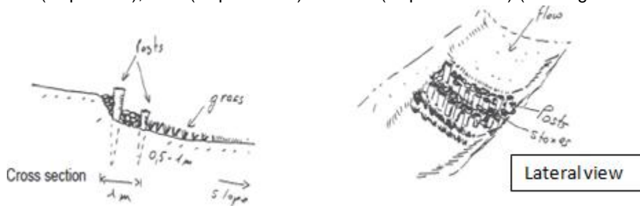
Figure 9: Check-Drop-Apron with wood posts and stones for vegetative waterways (Source: CBPWD guideline, 2005 )
