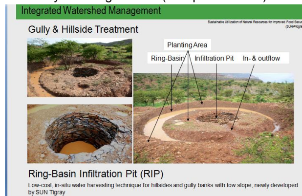
Photo : How percolation/infiltration pit is linked with ring-basin
