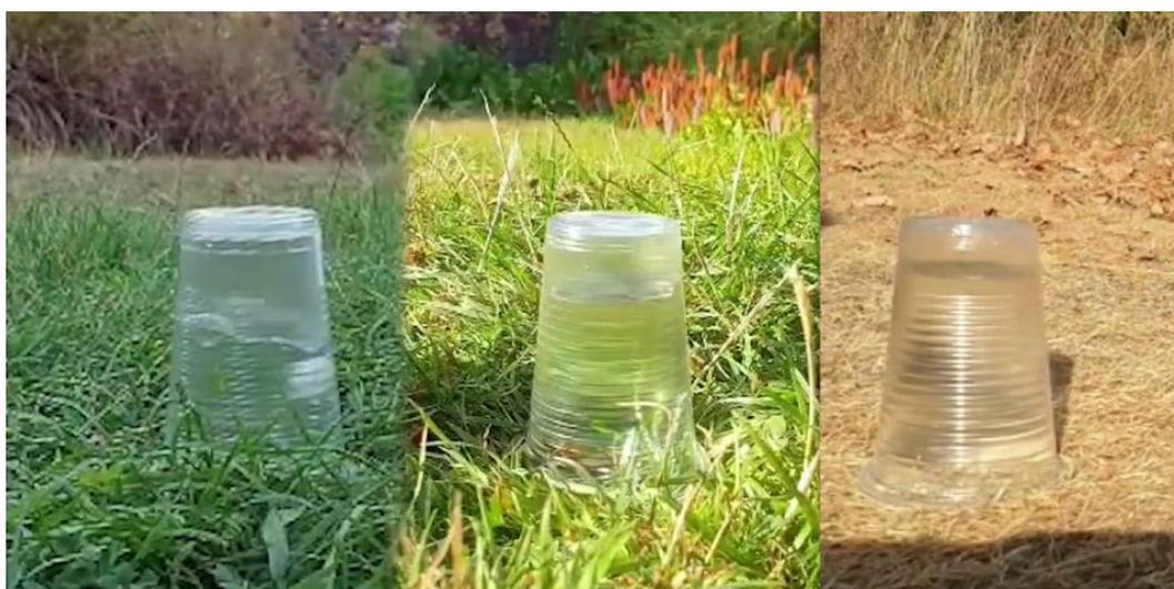
*Figure 1: Clip showing the effect of grass/crop cover on the infiltration rates.*
