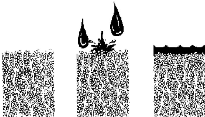
Fig. 22. Sealing of the soil surface by raindrops
