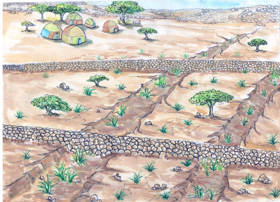
Illustration 5: Sequence of two dry-stone dams. Sediment and water infiltrate, enriching the land above and below the dry-stone dams
