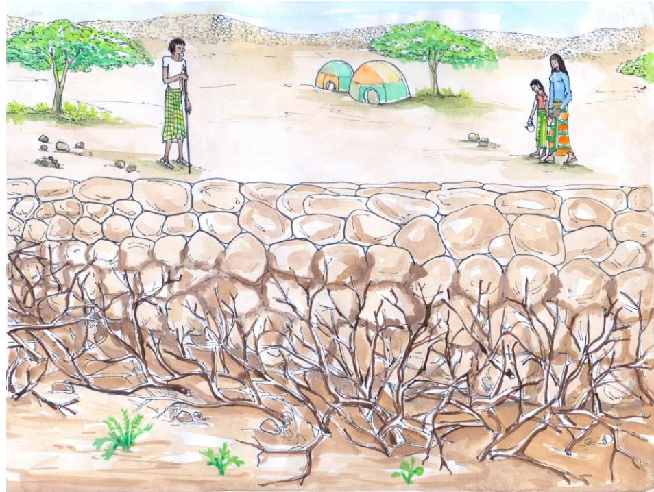
Illustration 6: organic matter will sediment and water infiltrates, enriching the land above and below the drystone structure
