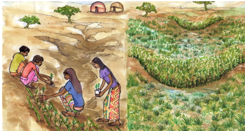
Figure 15: The first steps of the biological check dam and a fully grown and functional biological check dam
