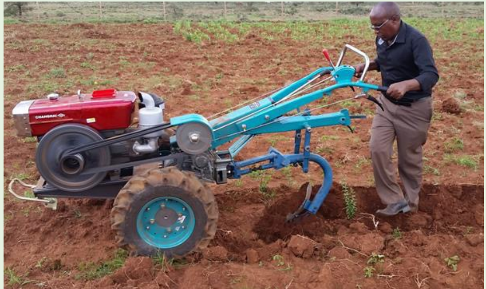
Single Axle Tractor in operation (source: Greentree)
