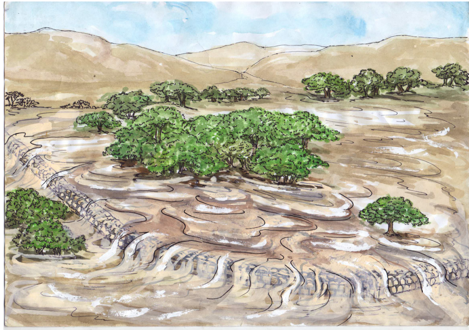
Figure 7: Water Spreading Weirs spread the water over a larger area, contributing to sediment deposition and build-up of shallow aquifers, as well as soil moisture in the top soils.
