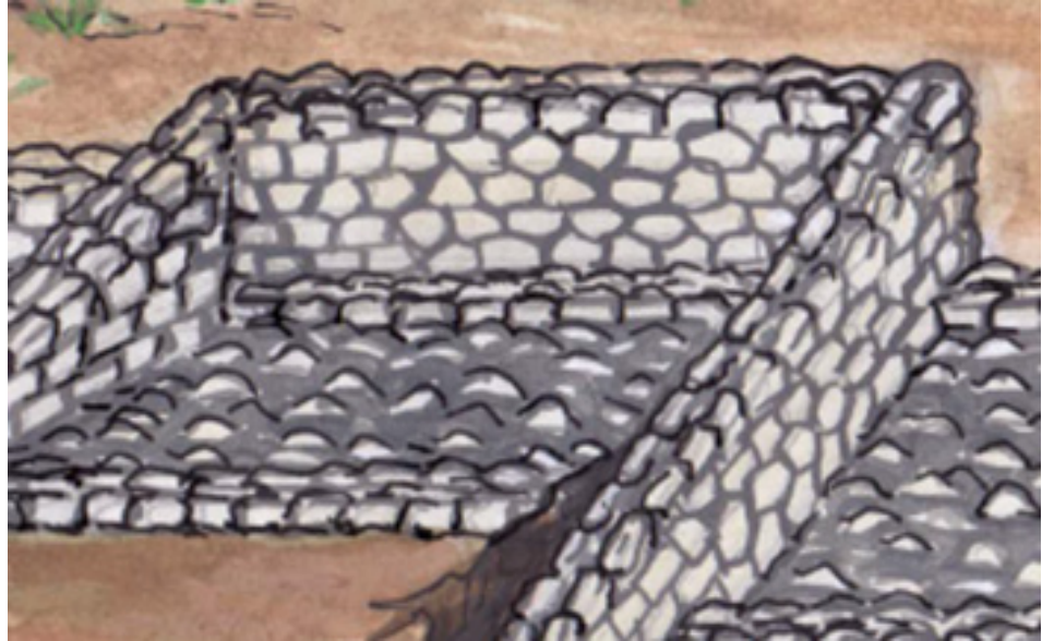
Figure 19: Constructed main wall of water spreading weir
