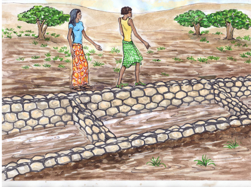
Figure 22: Counter wall and section division
